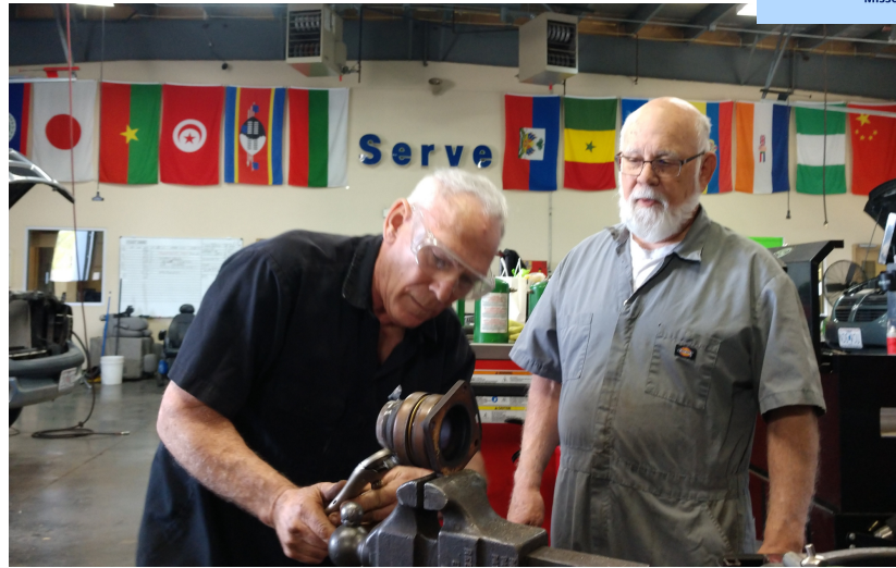
Mechanics Fred Tuggy and Chuck Hlavaty rebuild a catalytic converter
